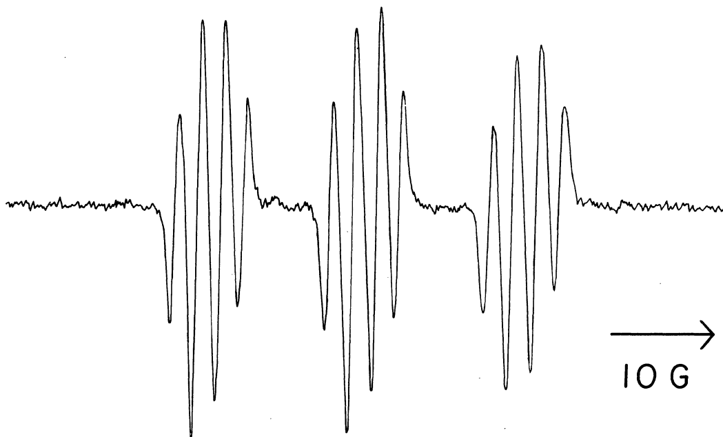
Figure 2. ESR spectrum of a \gamma -irradiated aqueous glycyglycine solution. The concentrations of glycyglycine and 2-methyl-2-nitrosopropane were 0.2 M and 0.05 M , respectively.
